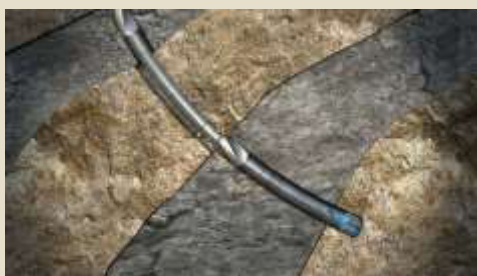
Example of Wellbore Geometry Stick: Stuck at a Ledge at High Angle
