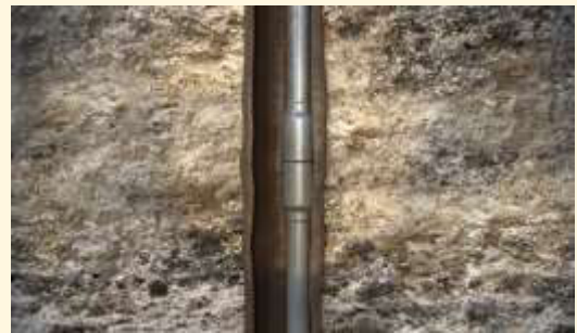
Differentially Stuck Drillpipe
